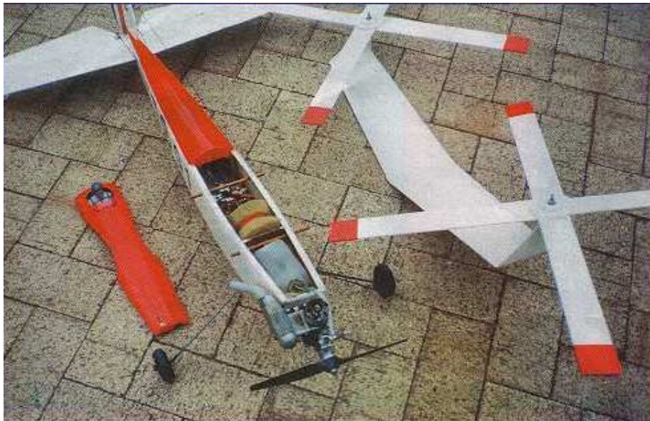
Tango Autogyro dismantled showing compact radio installation and fuel tank. Engine is an OS .40 two stroke.
