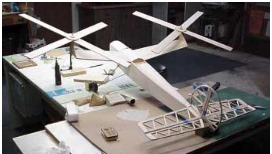
Red Scholefield's Tango. Bolt on wing, double strut 1/8 inch piano wire landing gear, built up tail surfaces, removable tank hatch, side mounted engine. Covered in monokote. Otherwise built to plan. 4 1/2 lbs. OS .40FP
