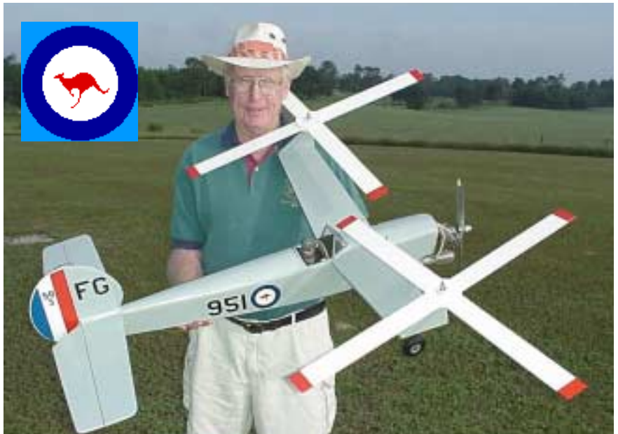
Red Scholefield's Tango. Bolt on wing, double strut 1/8 inch piano wire landing gear, built up tail surfaces, removable tank hatch, side mounted engine. Covered in monokote. Otherwise built to plan. 4 1/2 lbs. OS .40FP
